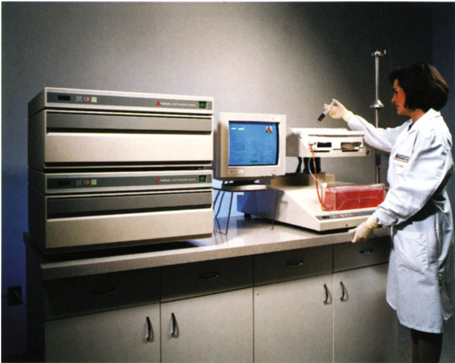
Fig. 4. Photograph of the prototype AASTROM cell-production system (CPS). The AASTROM CPS consists of the incubator(s) ( left ), system manager ( center ), and processor ( right ). A disposable cell cassette is being inoculated with cells as it sits on the processor platform
