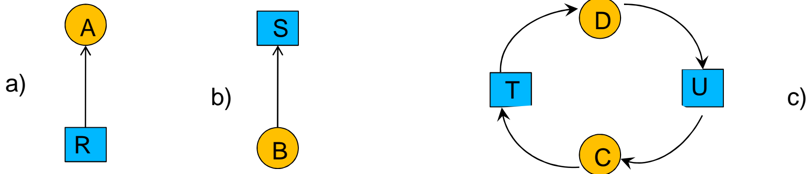
Resource allocation graphs. (a) Holding a resource. (b) Requesting a resource. (c) Deadlock
