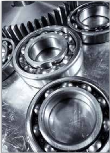
Ball bearings are used to reduce friction between moving machine parts.
