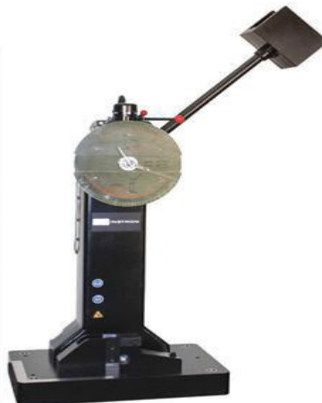
Fig. 7. Instrumented impact pendulum system for Charpy testing (courtesy of Instron)
