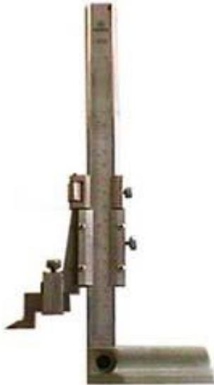
Figure62. vernier height gauge
