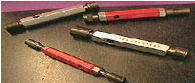
**Figure 70. Different size Plug gage**
