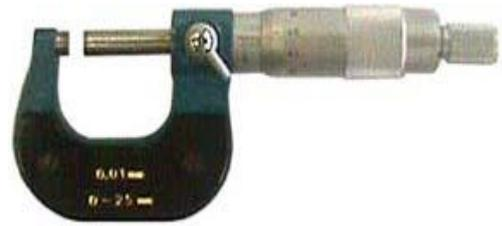
Figure 63. Outside Micrometer
