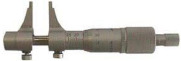
Figure 64. Inside Micrometer
