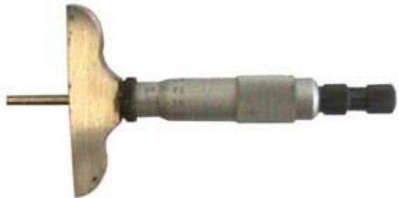
Figure 65. Depth Micrometer
