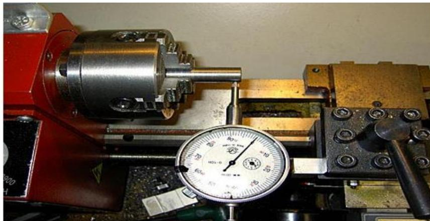
Figure13.center work in a 4-jaw chuck
