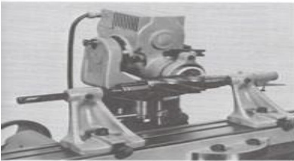
**Figure26. Grinding a plain milling cutter**
