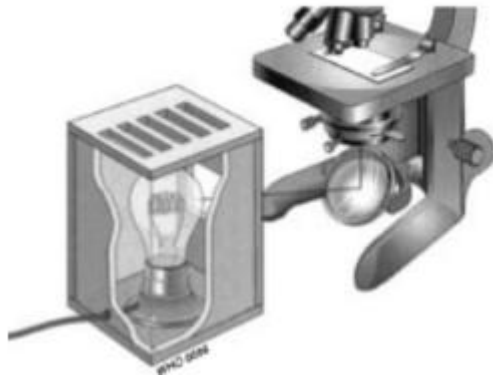
Fig. 3.7. Setting up a Lamp for a Microscope
