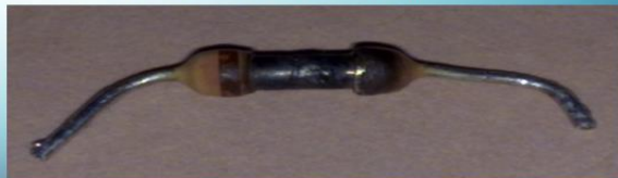
Physical appearance of bad/defective resistor
