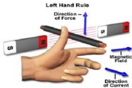
Fig. 5.2.2 Fleming Left Hand Rule
