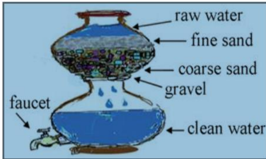
Figure 8.1: Household water filter using two clay pots placed on top of each other
