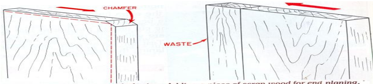
Chamfering an end for end planing. Adding a piece of scrap wood for end planing.
