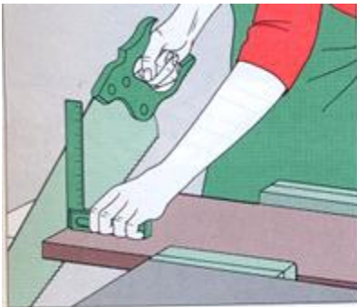
Checking a saw with a try square
