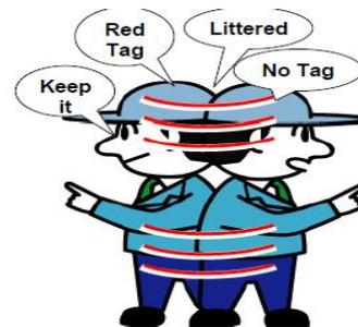
**Set in order:** is the 2<sup>nd</sup> of the five components of 5S. Set-in-order means deciding the place for necessary items, arrange them to keep easy access, and display signs so that they can be found immediately and returned or replenished properly.
