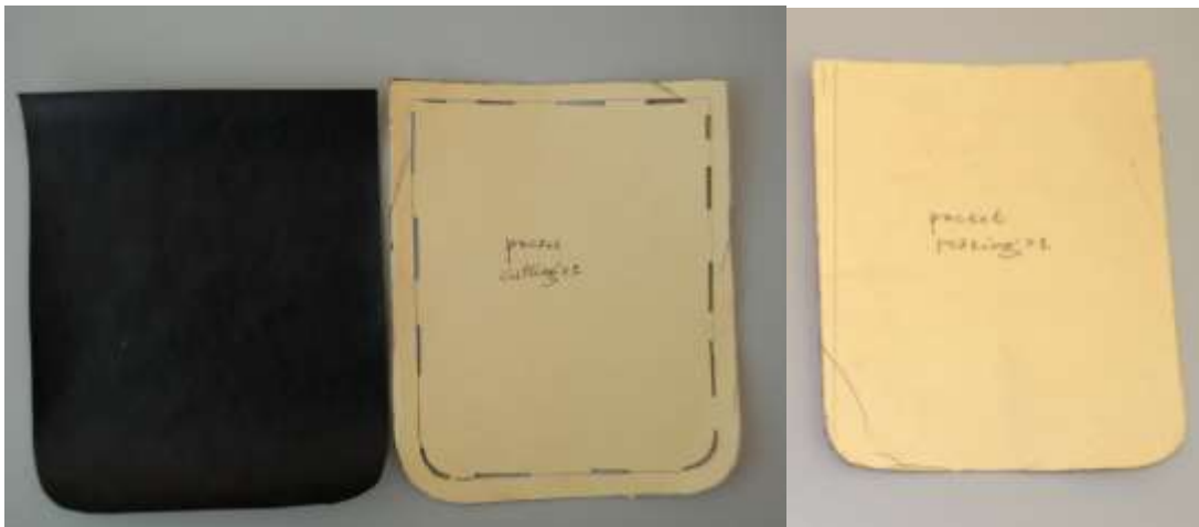
Figure: from right to left pocket making pattern, pocket cutting pattern and pocket component cut from synthetic leather
