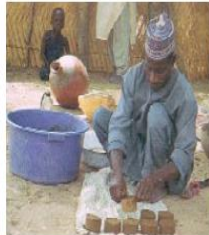
Removing molded blocks for drying
