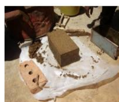
Step 5. UMB ready for drying
