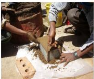
Step 3. Opening the mold
