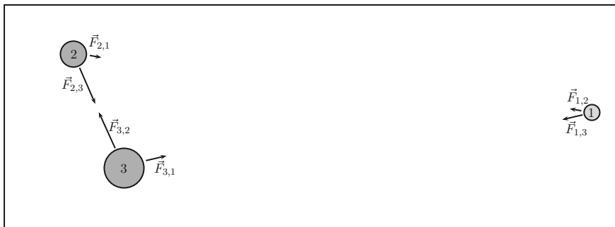
Fig. 1.1 Three massive bodies and the gravitational forces they exert on one another
