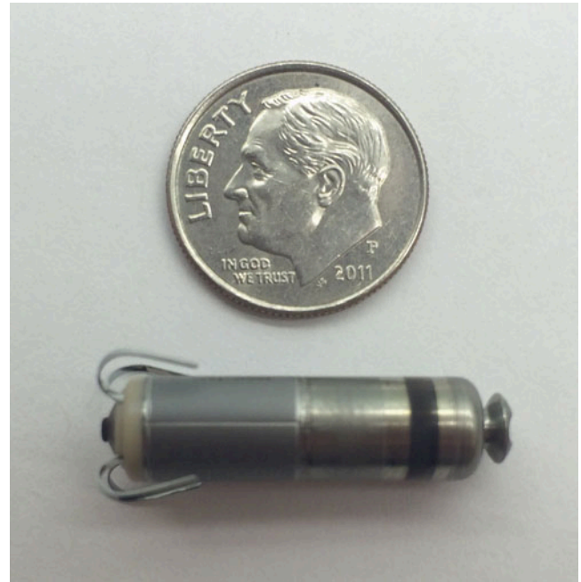
Fig. 30.44 Micra™ Transcatheter Pacing System (Medtronic, Inc., Minneapolis, MN, USA; not available for sale, but currently under clinical investigation)
