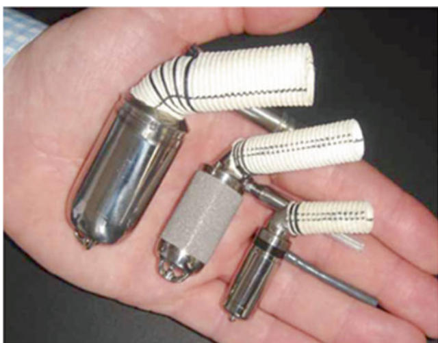
Fig. 11.8 Pediatric Jarvik 2000. This is an axial-flow blood pump designed to support patients in all size ranges; additionally it is implantable and provides chronic left, right, or biventricular support
