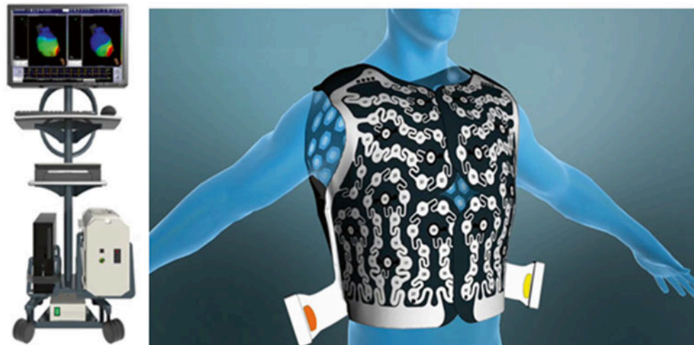
Fig. 32.13 ECVUE system and non-invasive vest. Image from http://www.cardioinsight.com/product/the-ecvue-vest-at-work/
