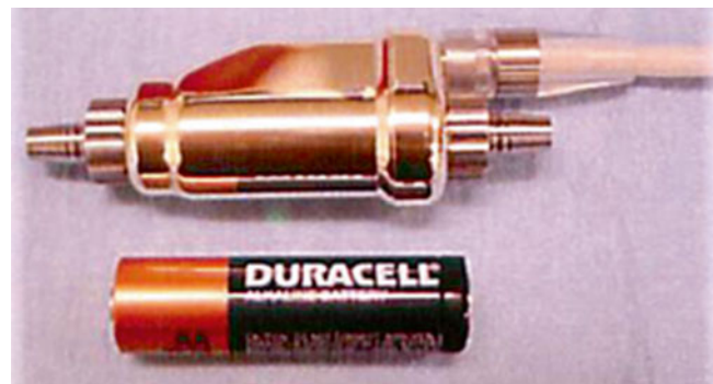
Fig. 11.7 PediaFlow ventricular assist device. This is an implantable, magnetically suspended mixed-flow turbodynamic blood pump to provide chronic circulatory support to patients from birth to 2 years of age with congenital or acquired heart disease
