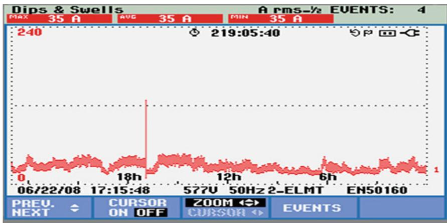
Fig. 8.27 Tripping of WM due to sag
