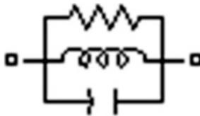
The Parallel RLC Load block implements a linear load as a parallel combination of RLC elements. At the specified frequency, the load exhibits a constant impedance. The active and reactive powers absorbed by the load are proportional to the square of the applied voltage.
