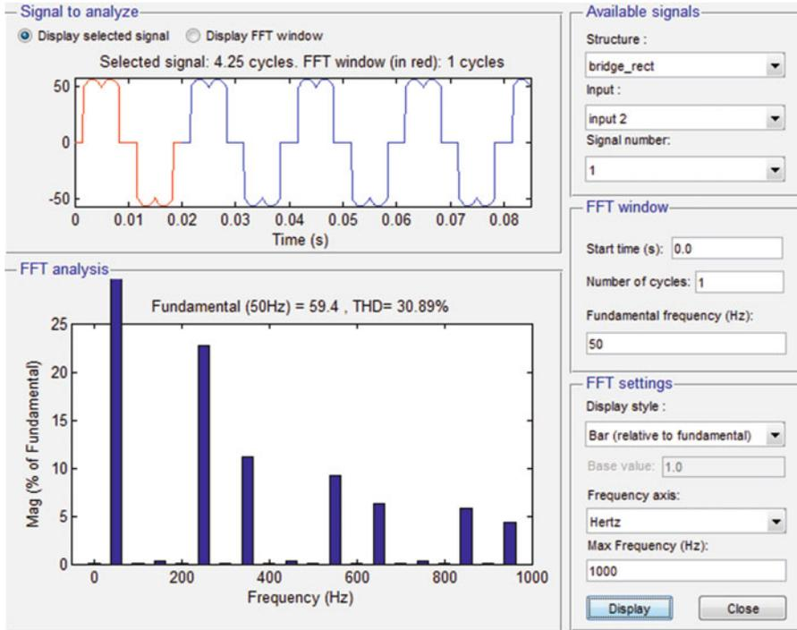
Fig. 6.60 THD analysis of source current in AC-DC rectifier
