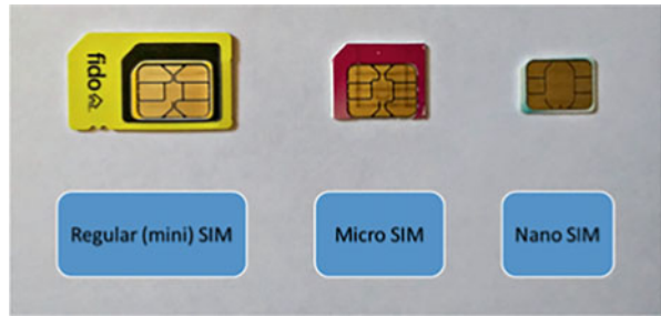
Fig. 17.2 Different sizes of SIM cards
