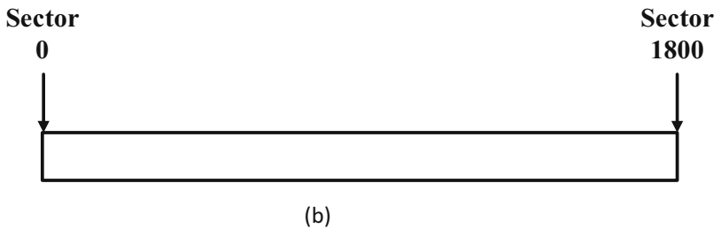
Fig. 4.1 Hard disk geometry. (a) Cylinder-head-sector. (b) An example of disk volume with size of 1801 sectors (or 1801X521 Bytes)
