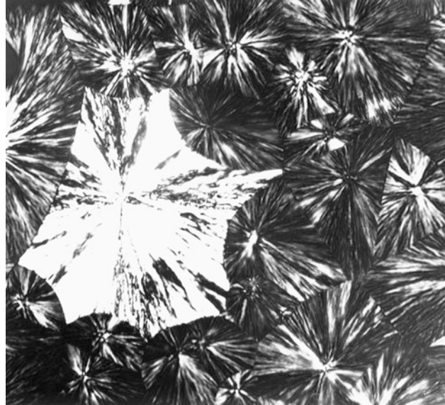
■ Fig. 5.9 Isotactic polypropylene viewed through a polarizing microscope (dark regions: \alpha -spherulite, light regions: \beta -spherulite)
