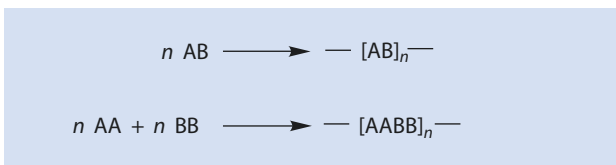
■ Fig. 8.6 A scheme of a step-growth polymerization
