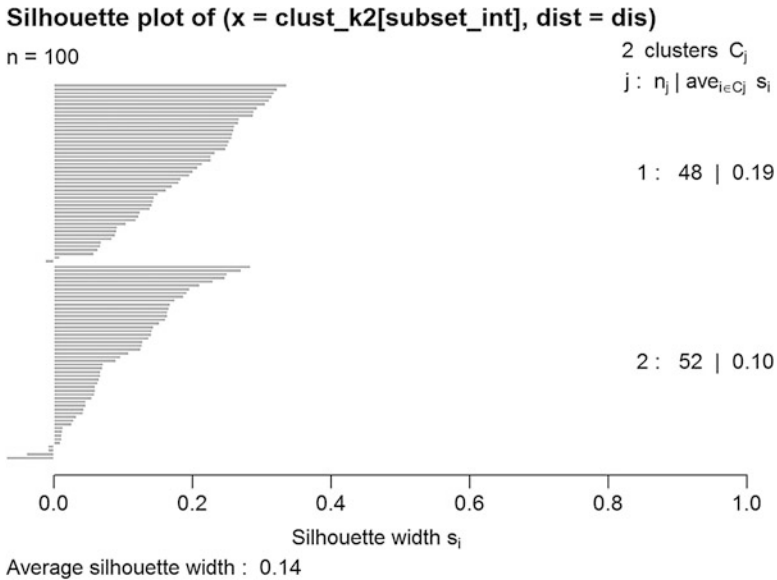
Fig. 21.8 Silhouette plot of the 2-class k-means clustering of the Parkinson's disease data
