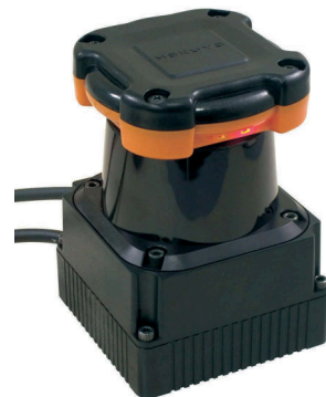
Fig. 6.6. A scanning laser range finder. The sensor has a rotating assembly that emits pulses of infra-red laser light and measures the time taken for the reflection to return. This sensor has a maximum range of 30 m and an angular range of 270 deg. Angular resolution is 0.25 deg and the sensor makes 40 scans per second (Courtesy of Hokuyo Automatic Co. Ltd.)
