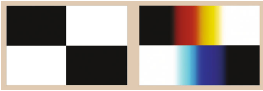
Fig. 11.20 There are two types of border colours, depending on which page is black and which is white in relation to the prism orientation. The left part of the figure shows the black and white distribution of light we start with. The right part shows how the image of the original light distribution would look if the light went through a prism. The colour effect is a simulation customized visual impression from a computer screen. Real reds look prettier, but they must be experienced in vivo !
