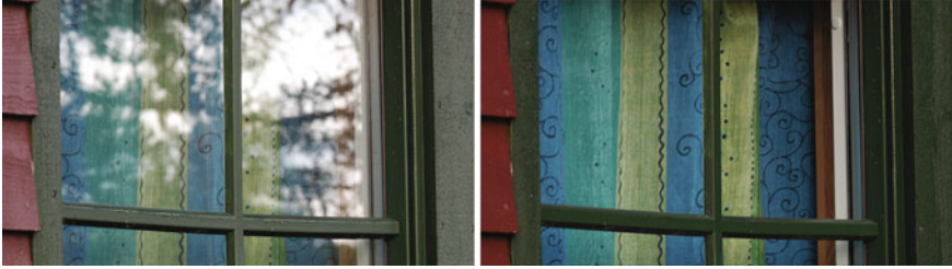
Fig. 10.7 Unpolarized light reflected at an air–glass interface can be fully polarized when the angle of incidence is equal to the Brewster angle. These photographs show this. The picture on the left is taken without a polarization filter. The picture on the right is taken with a polarization filter oriented so as to let only light polarized parallel to the incidence plane. All reflection is removed at the Brewster angle, and we look directly at the curtains behind the glass window practically without any reflection. This means that, at the Brewster angle, all the reflected light is fully polarized in a direction perpendicular to the incidence plane (parallel to the air–glass interface). Note that reflections on the painted surface are affected similarly to reflections from the glass. NB: Many modern windows are now surface treated in different ways. Then, we do not get any direct interface between air and glass, and the Brewster effect as described disappears totally or in part
