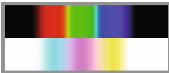
Fig. 11.21 Colour spectrum we get from a Newtonian column and the colour spectrum we get from a "reverse slit", i.e. a black narrow stripe on a light background. Also this picture is the result of a simulation. Real spectra (without going through photography or computer monitors) are far more beautiful to look at!
