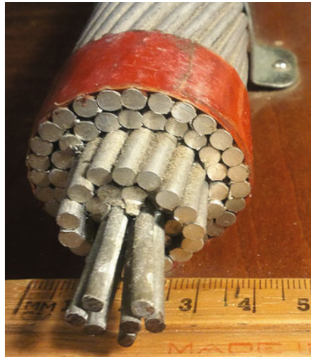
Fig. 16.9 Cross section of a type of conductor used in power lines hanging between large masts across large parts of the country. Clark Mills , Wikimedia Commons, CC BY-SA 3.0 , [3]
