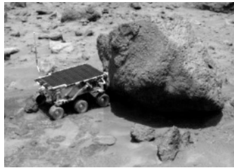
Fig. 1.35. The Sojourner rover was deployed by the Pathfinder lander and explored 250 m 2 of Martian soil in 1997 (courtesy of NASA)
