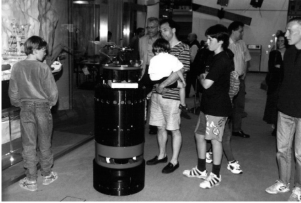
Fig. 1.38. Rhino, employing the synchro-drive mobile base B21 by Real World Interface, was one of the first robots for museum guided tours (courtesy of Deutsches Museum Bonn)
