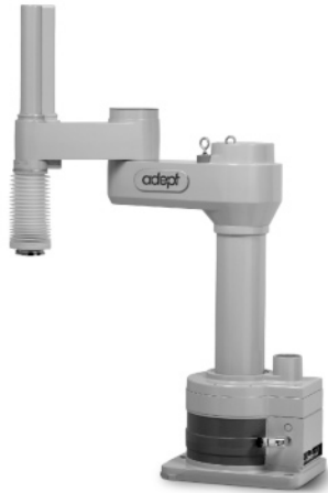
Fig. 1.24. The AdeptOne XL robot (courtesy of Adept Technology Inc)
