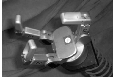
Fig. 1.31. The BarrettHand (courtesy of Barrett Technology Inc)
