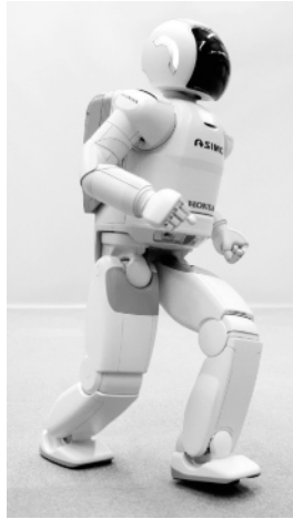
Fig. 1.41. The Asimo humanoid robot, launched in 1996, has been endowed with even more natural locomotion and human-robot interaction skills (courtesy of Honda Motor Company Ltd)
