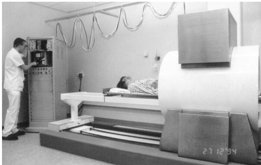
Figure 9.3 The whole-body counter of University Medical Centre, Utrecht, The Netherlands. The counter has a mobile shadow shield with two NaI(Tl) scintillation detectors (4 × 6 in) placed at opposite sites of the subject. The lead shielding is 100 cm long with a diameter of 90 cm. The scanner moves on rails over a distance of 240 cm with an adjustable speed. Extreme variations in geometry yield practically the same value for ^{59}\text{Fe} activity. The equipment can be used for measurements in man and small animals.
