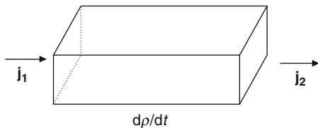
Fig. 4.1 Conservation of probability density. The rate of change within a certain interval is given by the flux differences at the boundaries of the interval
