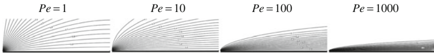
Fig. 3.15 Isotherms at increasing values of Péclet number for fluid flow over a flat plate maintained at a hot uniform temperature
