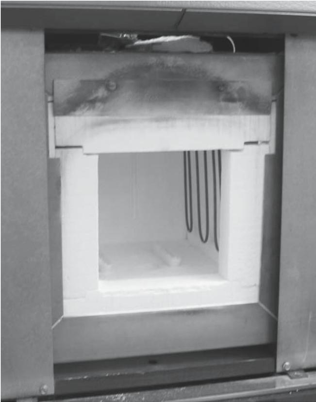
**FIGURE 9.2** A small electrically heated box furnace.
