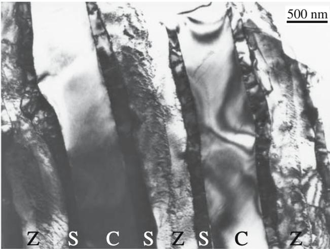
**FIGURE 15.18** A CoO/ZrO<sub>2</sub> eutectic after solidification and subsequent oxidation. Z, ZrO<sub>2</sub>; C, CoO; S, Co<sub>3</sub>O<sub>4</sub> (spinel).
