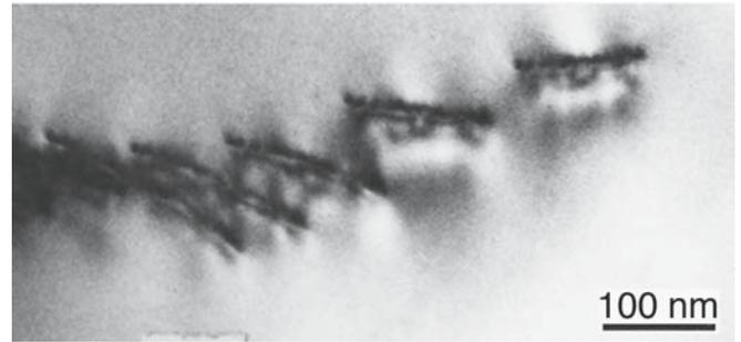
FIGURE 12.8 Diffraction contrast from dislocations in  $\text{Al}_2\text{O}_3$ .
