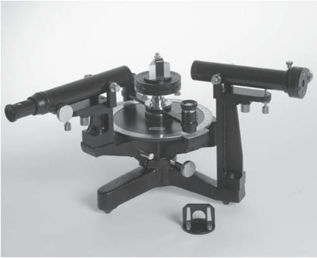
FIGURE 36.7 Goniometer-style refractometer.
