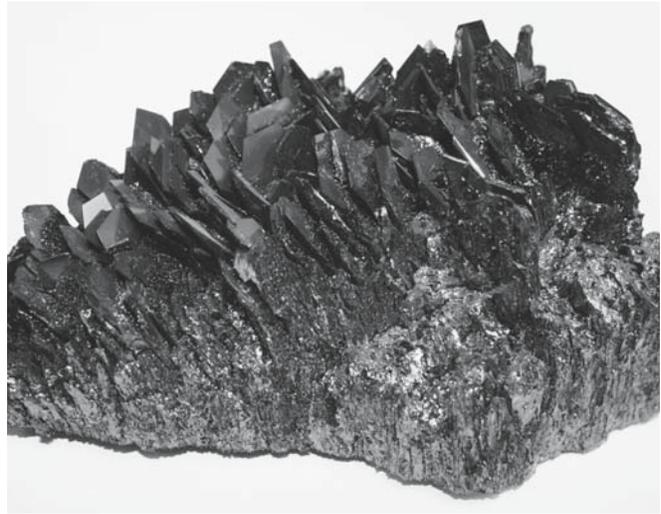
FIGURE 19.7 SiC produced by the Acheson process.
