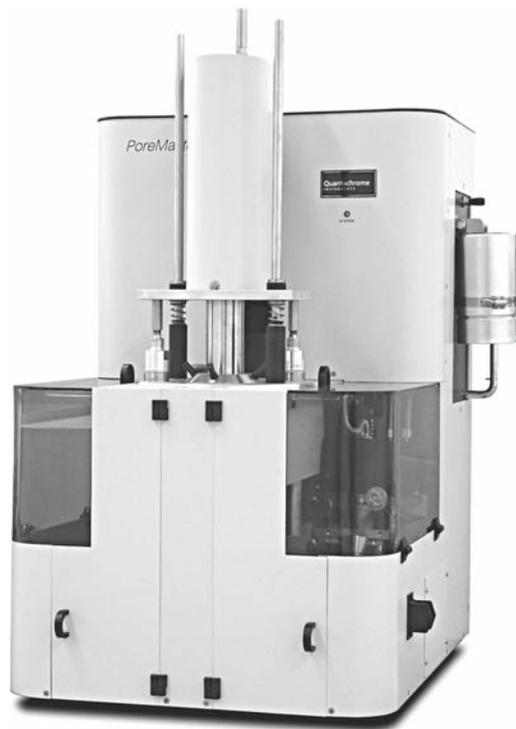
FIGURE 15.13 A commercial porosimeter.
