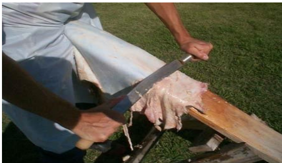
Figure 10. Fleshing using a fleshing knife
