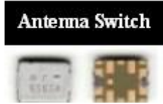
Fig. 2.25 Shows Antenna Switch of Mobile Phone
