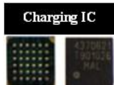
Fig. 2.33 Shows Charging IC of a Mobile Phone
