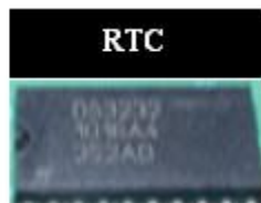
Fig.2.22Shows Mobile Phone RTC (Real Time Clock)
