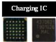
Fig. 2.21 Shows Cell Phone Charging IC
