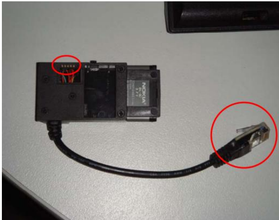
Fig4.8 Connectors on the UFS3 cable for Nokia 6600
