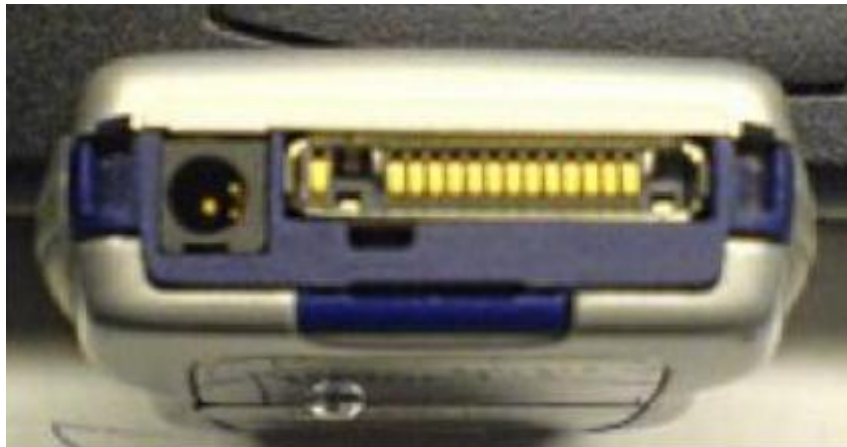
Fig 4.9 Nokia 3220 Fbus connections (Harrington 2007)
