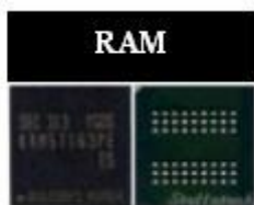
Fig. 2.18 Shows Mobile Phone RAM
