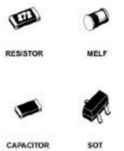
Fig 5.6 - Common discrete SMT components
