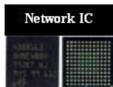
Fig. 2.12 Cell Phone Network IC / RF IC
