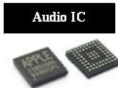
Fig. 2.22 Shows Cell Phone Audio IC Called Cobba IC and Melody IC.
