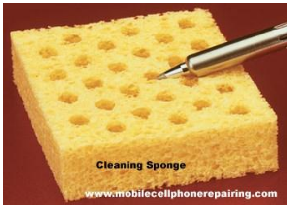
Fig.2.24 Shows Cleaning Sponge to Clean Tip of Soldering Iron
