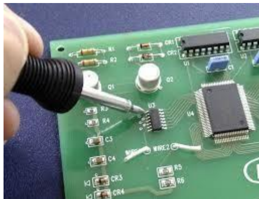
Fig2.2. Picture showing A technician Soldering
