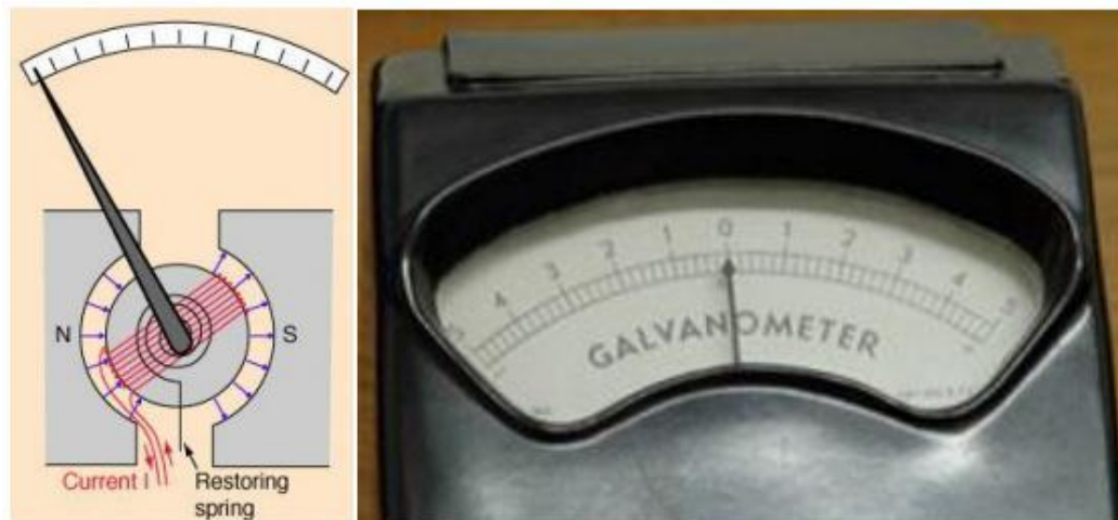
Fig4.6. Schematic and photograph of a Galvanometer used for sensing electrical currents
