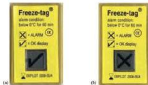
Figure 6.9 Freeze-tags showing: (a) 'good status' display; (b) 'alarm status' display.
