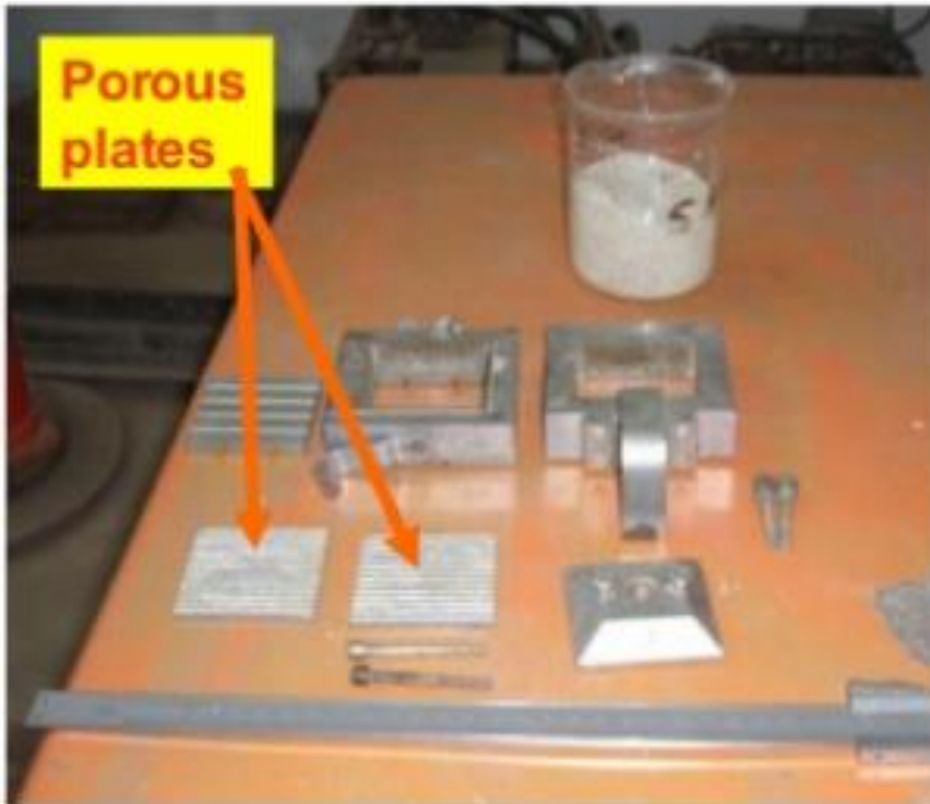
Components of the shear box
