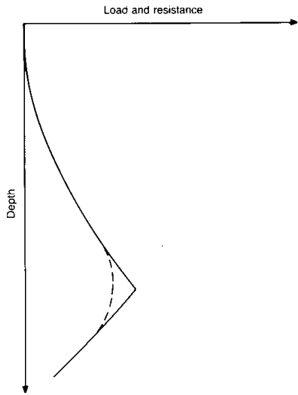
Fig. 3. Residual load present in the pile immediately before the start of the static loading test
