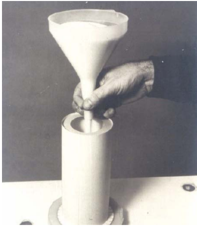
Loading model silo – note temporary former Paper silo: radial displacements at top due to 10 percent eccentric discharge from 2/3 radius
