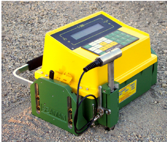
Figure 5.9 Nuclear density meter. (Photo courtesy of Seaman Nuclear Corp.)
