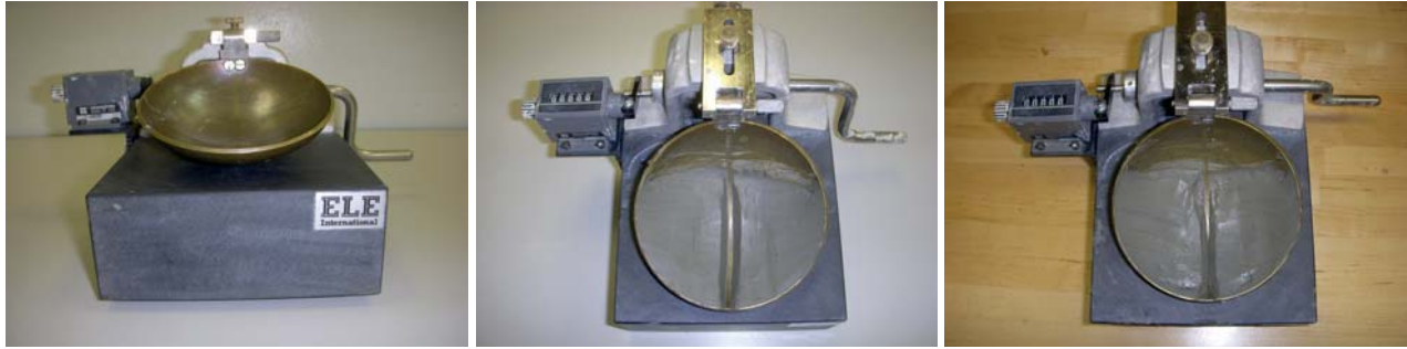
Figure 4.9 Liquid limit apparatus and test.
