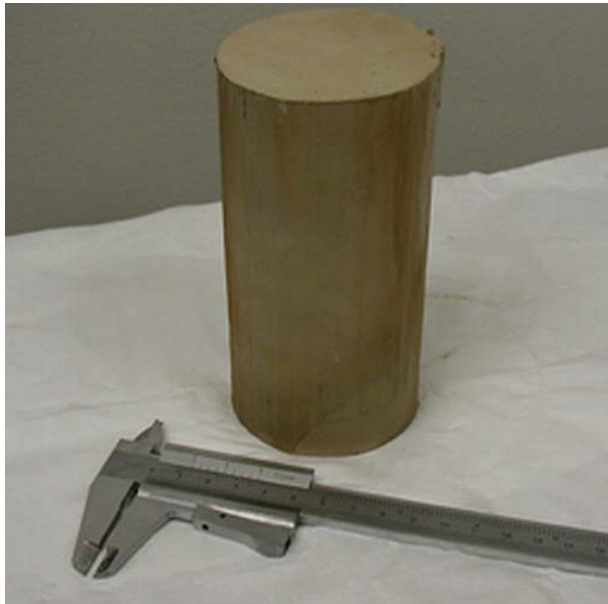
Figure 4.14 Free shrink test for shrinkage limit of undisturbed sample.
