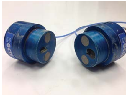
Figure 9.16 Bender elements: (a) Principle. (b) Device.
