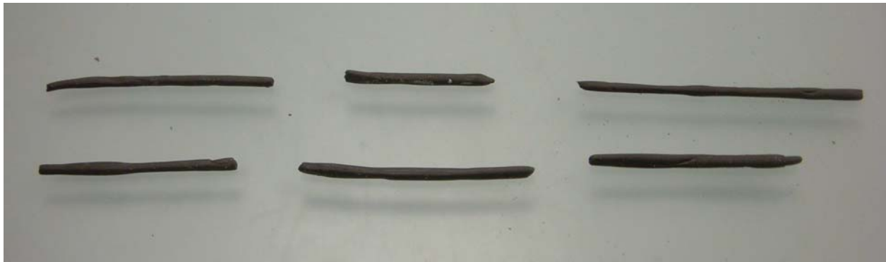
Figure 4.10 Plastic limit test and soil threads.
