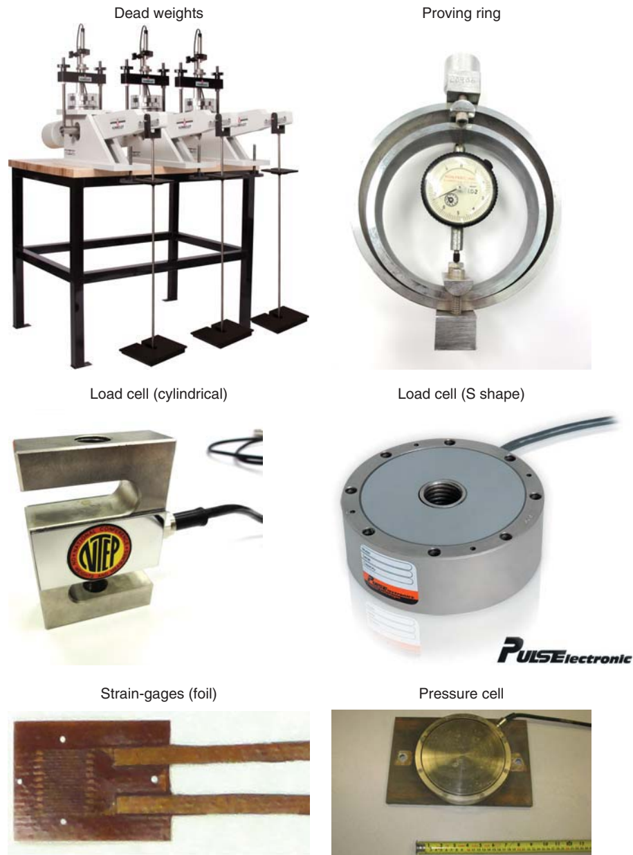
Figure 9.2 Devices to measure normal stress. (a) Dead weights. (b) Proving ring. (c) Load cell (S shape). (d) Load cell cylindrical. (e) Strain gages (foil). (f) Pressure cell. (a: Courtesy of Humboldt Mfg. Co.. d: Courtesy of Mediscale1.)
