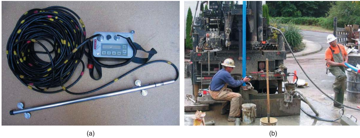
Figure 19.44 Inclinator instrument and casing installation. (a) Inclinator. (b) Casing installation. (Courtesy of Landslide Technology.)
