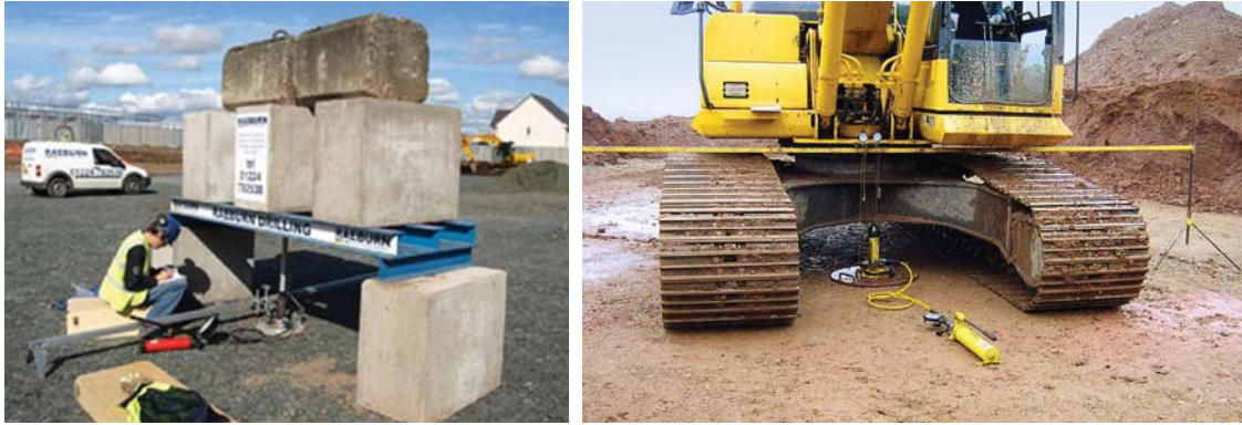
Figure 7.25 Plate load tests. (a: Photo by David Wilkins. Courtesy of Raeburn Drilling and Geotechnical (Northern) Limited; www.raeburndrillingnorthern.com . b: Courtesy of GEMTECH Limited, Fredericton, New Brunswick.)
