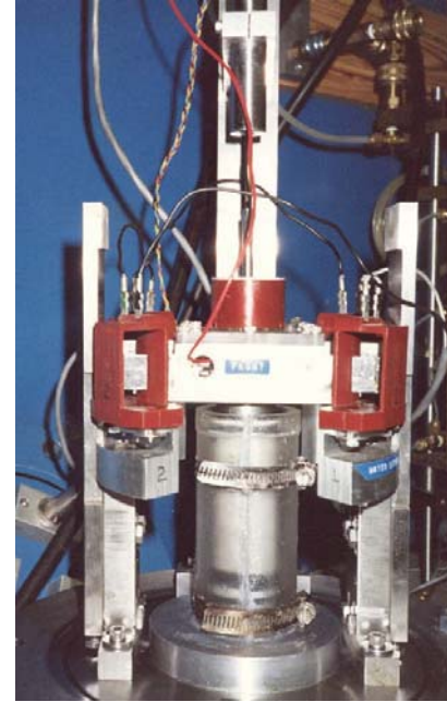
Figure 9.55 Resonant column test: (a) Principle. (b) Equipment. (b: Courtesy of Geotechnical Research Lab, Dept. of Civil Engineering, University of British Columbia.)
