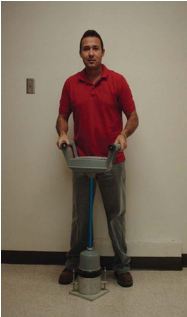
Figure 20.6 BCD-Proctor laboratory compaction test for modulus determination.
