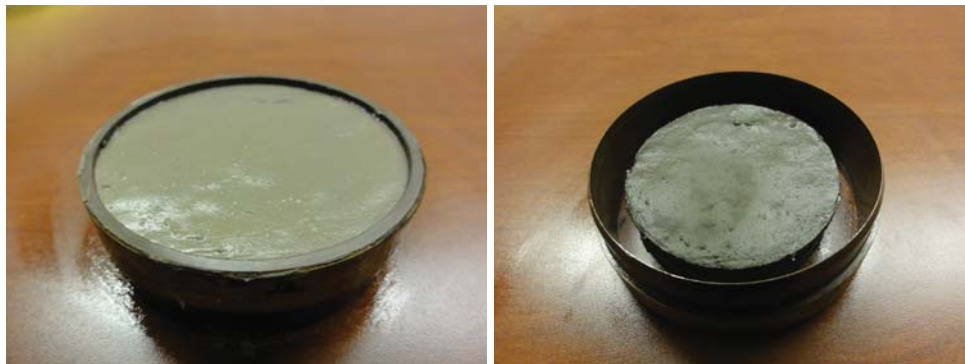
Figure 4.11 Shrinkage limit equipment and test.
