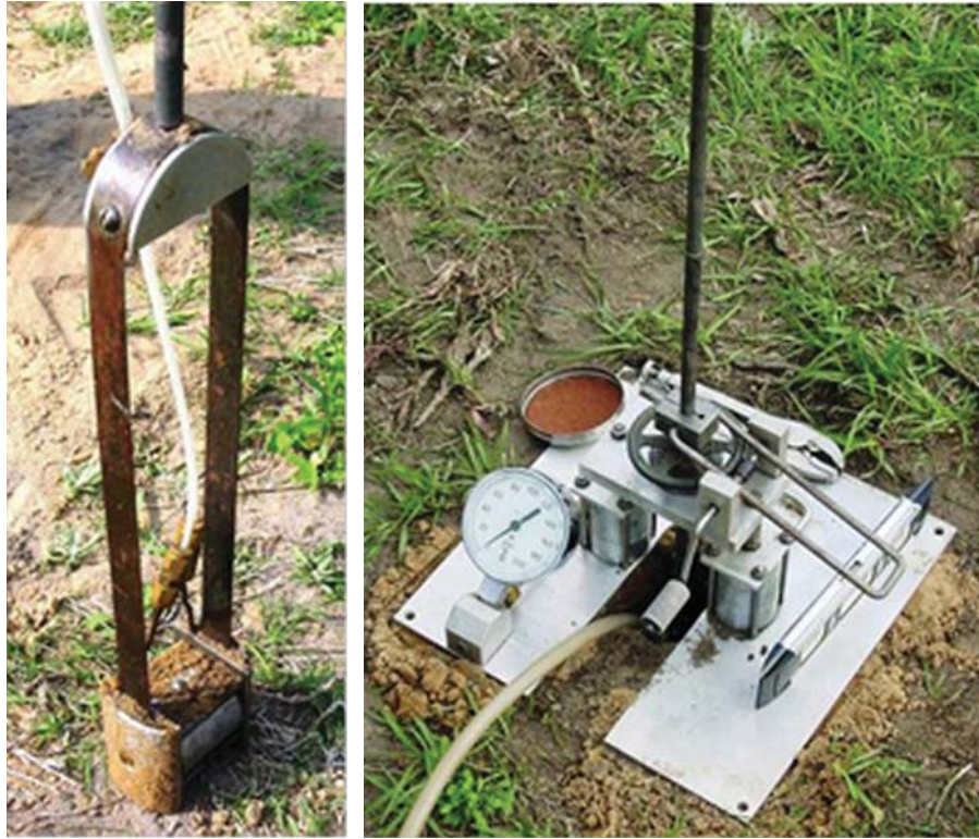
Figure 7.22 Borehole shear test device. (Courtesy of In-Situ Soil Testing, L.C.)
