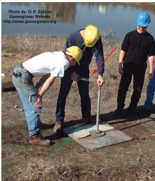
Figure 7.19 Field vane shear test. (Courtesy of Dr. Dimitrios P. Zekkos.)
