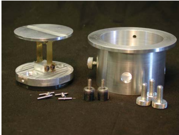
Figure 9.3 Shear stress sensor. (Courtesy of Department of Mechanical Engineering, University of Idaho, USA)
