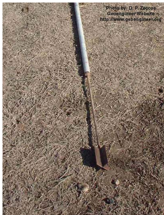
Figure 7.19 Field vane shear test. (Courtesy of Dr. Dimitrios P. Zekkos.)
