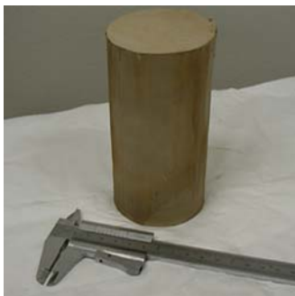
Figure 9.37 Free shrink test for shrinkage limit of undisturbed sample.
