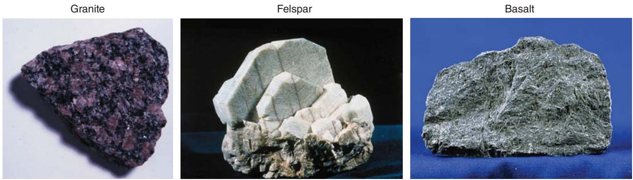
Figure 5.1 Igneous rocks: (a) granite, (b) feldspar, (c) basalt. (Courtesy of Mineral Information Institute, an affiliate of the SME Foundation.)
