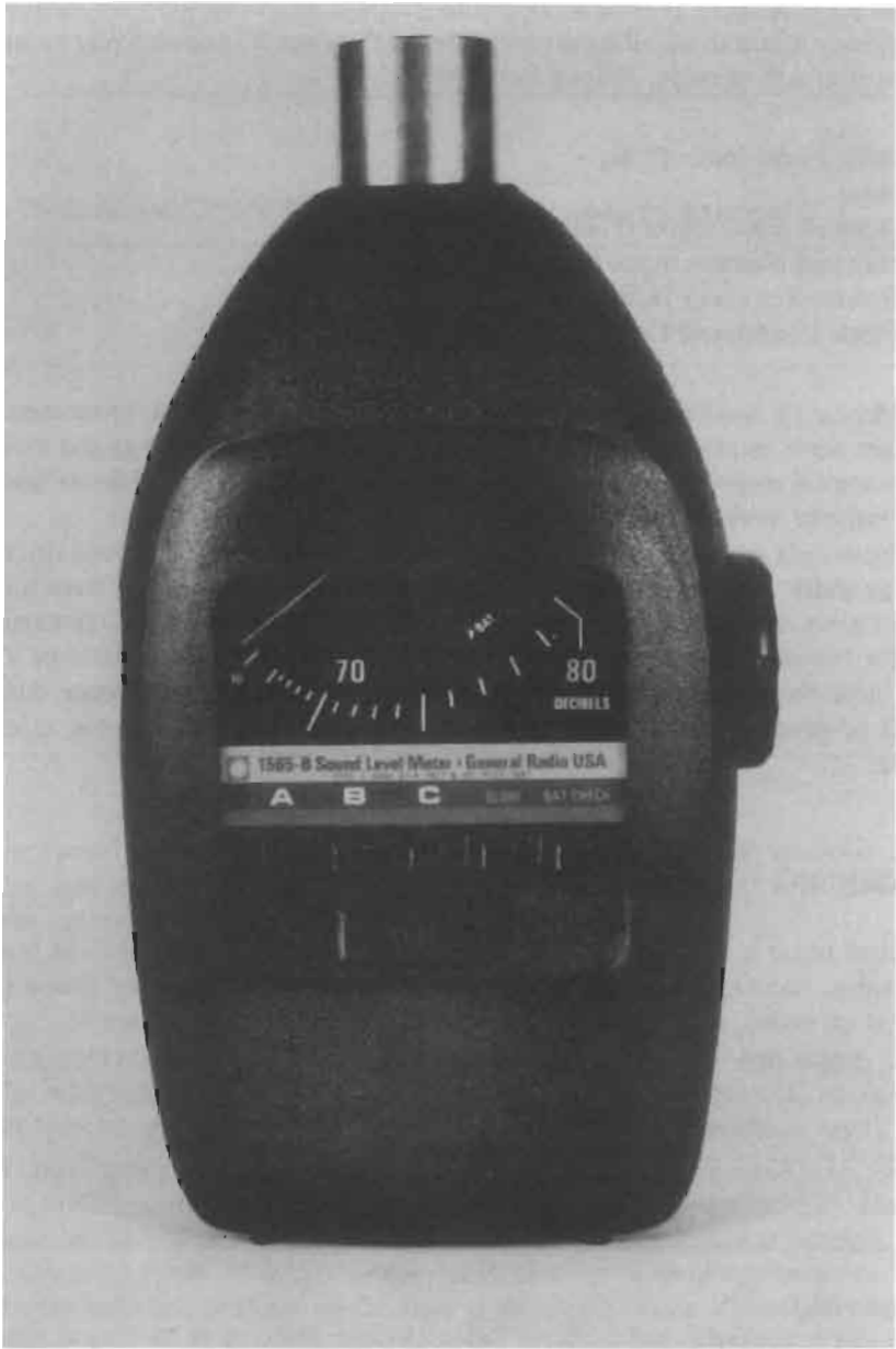
Figure 22-8. A typical sound level meter. (Courtesy of General Radio.)
