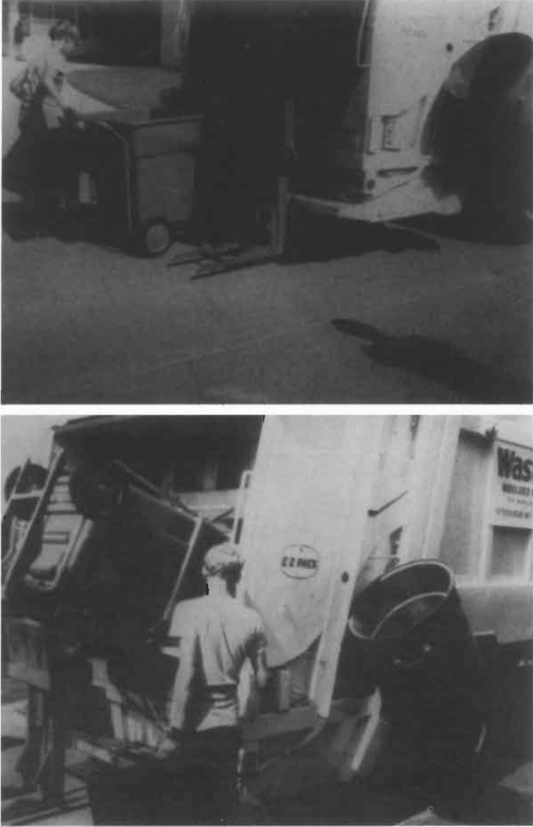
Figure 12-5. The “green can” system of solid waste collection.
