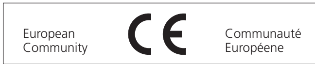
Figure A.2. The EC mark, signifying a product complies with the relevant standard or technical approval
