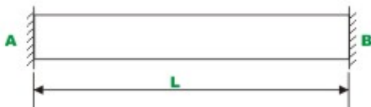
Fig. 9.4 Fixed - fixed beam
