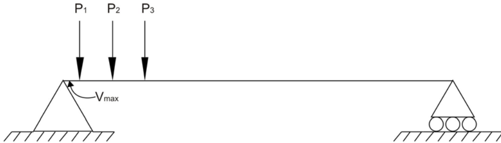
Figure 39.23: Absolute maximum shear – simply supported beam
