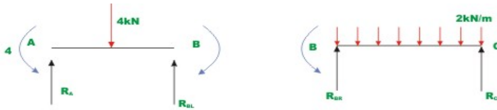
Fig.13.2 (c) Free - body diagram of two members
