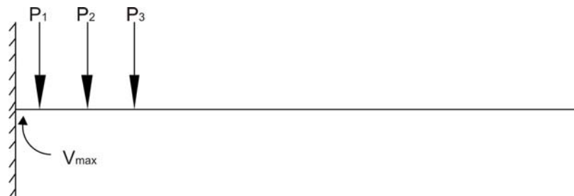
Figure 39.22: Absolute maximum shear case – cantilever beam
