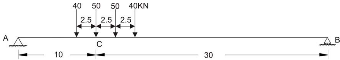
Figure 39.18: Beam loaded with a series of loads – Second load at section C
