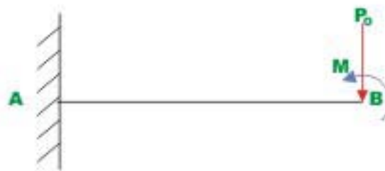
Fig.23.3(a) Cantilever beam
