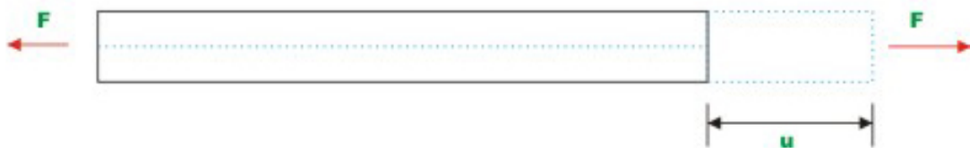
Fig 24.2 Force - displacement relationship
