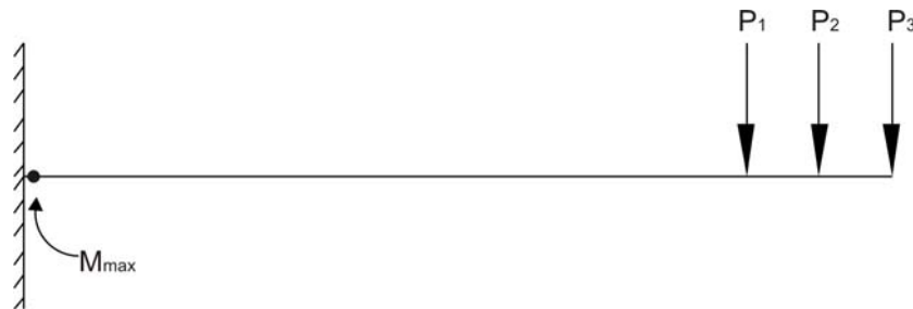
Figure 39.24: Absolute maximum moment – cantilever beam
