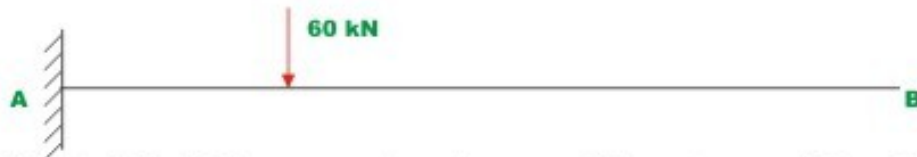
Fig. 7.6b Primary structure with external loading
