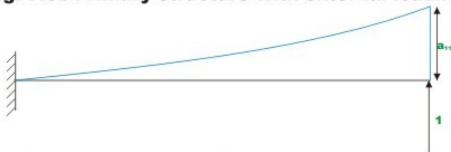
Fig. 7.6c Primary structure with unit load applied along R_B
