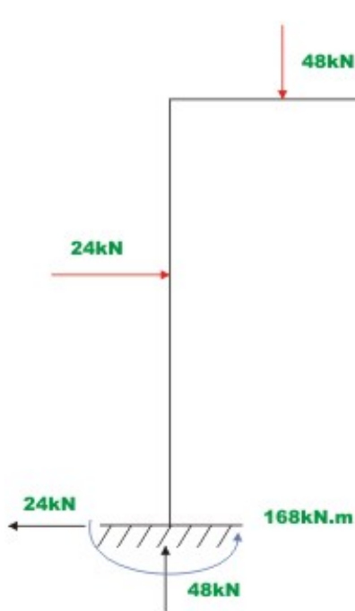
Fig 11.3 (b) Primary Structure
