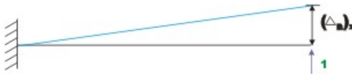
Fig. 7.2(d) Cantilever beam with a unit value of load along redundant R_b
