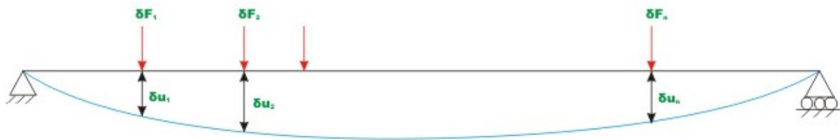
Fig. 5.1b : virtual system of forces.
