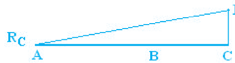
Figure 3.1c - Influence line for the reaction at support C
