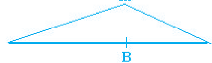
Fig 3.1g Influence line for Bending moment at point B.
