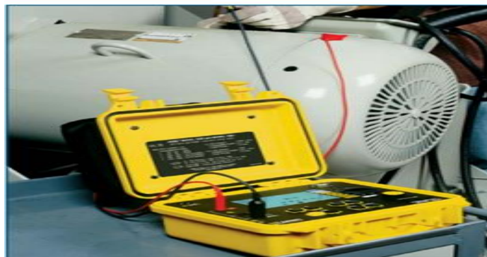
Fig.1.21. Measuring insulation resistance
