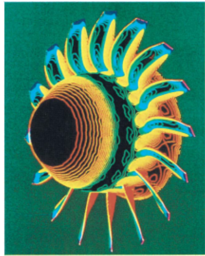
Plate 5 Density distribution on rotating fan blades and spinner, outer diameter 450 mm, speed of rotation 12 700 rpm (blue: low, red: high) (finite difference method) (page 289)
