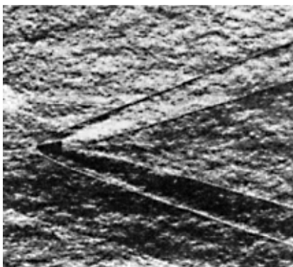
Fig. 13.7 Cone flying at supersonic velocity (Schlieren method) in air, Mach 3
