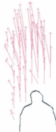
Plate 12 Natural convection around a human body (density correlation method). Maximum ascending velocity is about 0.2 m/s (page 286)
