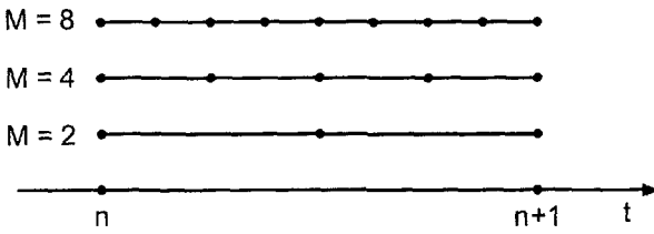
Figure 7.15 Grids for the extrapolated modified midpoint method.
