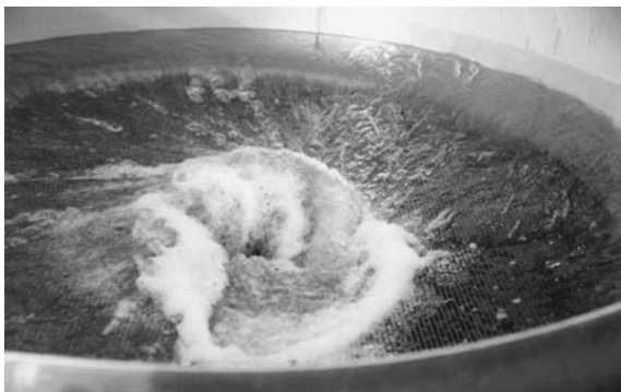
Fig. 12.10 Self-cleansing screen: Swirl-Cleanse™ Screen (courtesy of Hydro International)
