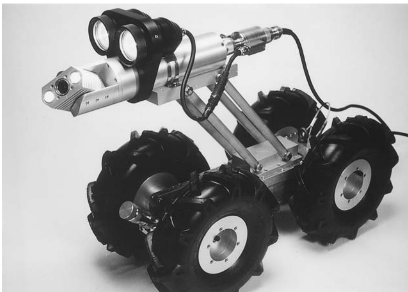
Fig. 17.3 A pan and tilt in-sewer CCTV camera (courtesy of Telespec Ltd, Guildford)
