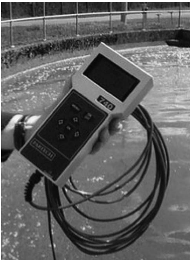
Fig. 1.1 – Portable suspended solids monitor (courtesy of Partech, UK)
