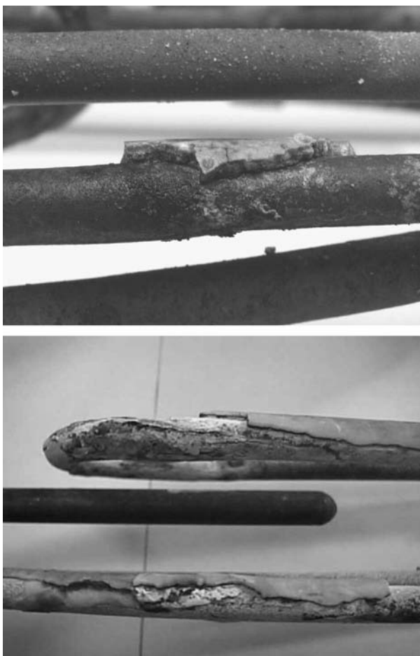
Fig. 4.19 – Examples of scaling and corrosion on heater elements
