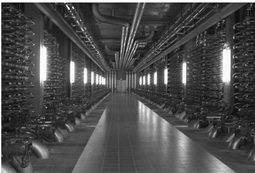
Fig. 7.13 – A potable water nanofiltration plant (courtesy of Viola, France)
