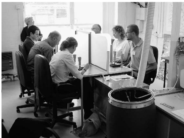
Fig. 9.1 – Olfactometry panel (courtesy of Silsoe Research Institute, UK)
