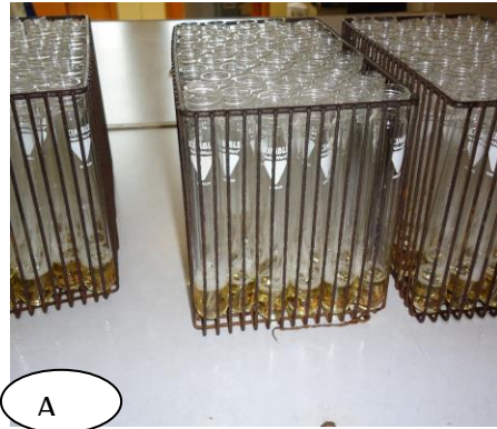
Fig3.2 A) Lactose broth used for total coliform count B) BGB fecal coliform count For physico chemical water quality determination the following reagents were used
