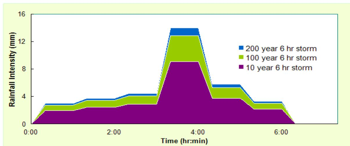
**Figure 33: Six hours design storm hyetographs used for rainfall - runoff modeling**
