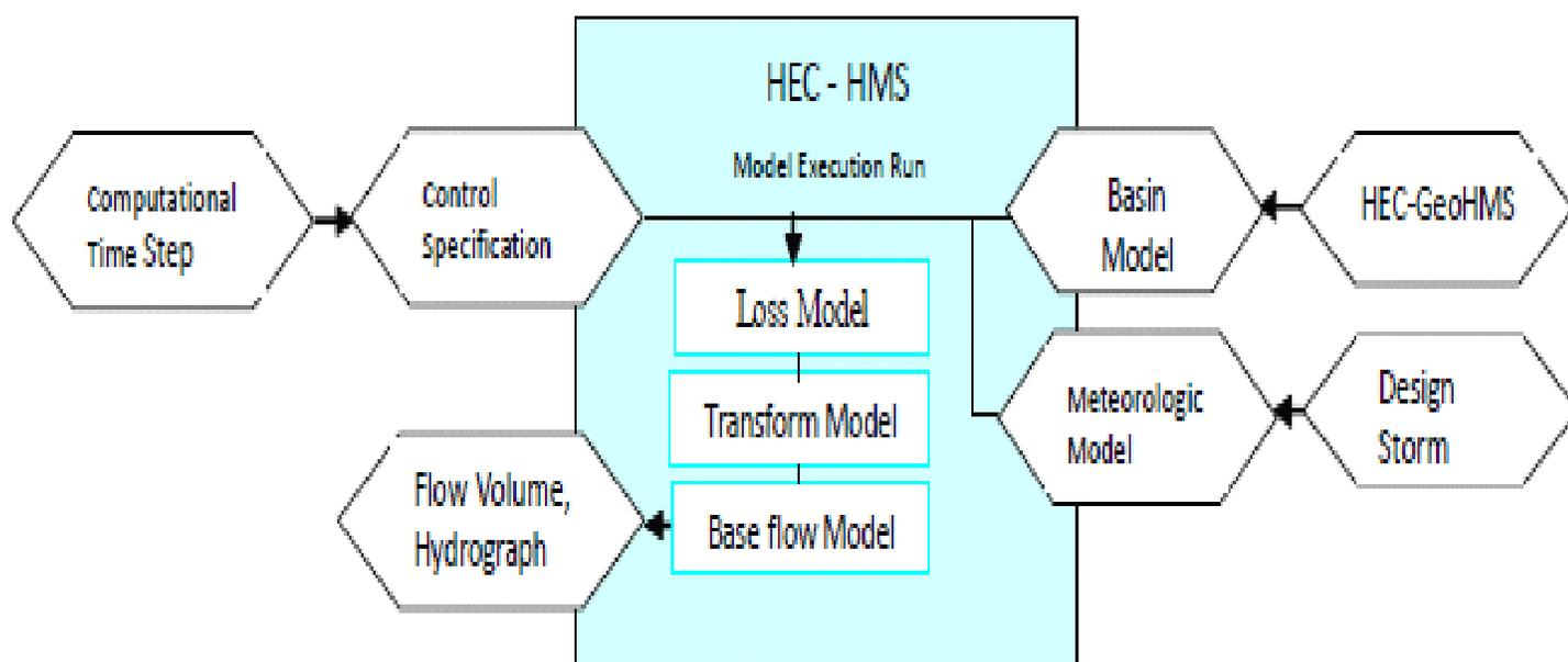
**Figure 16: HEC - HMS Software Components**
