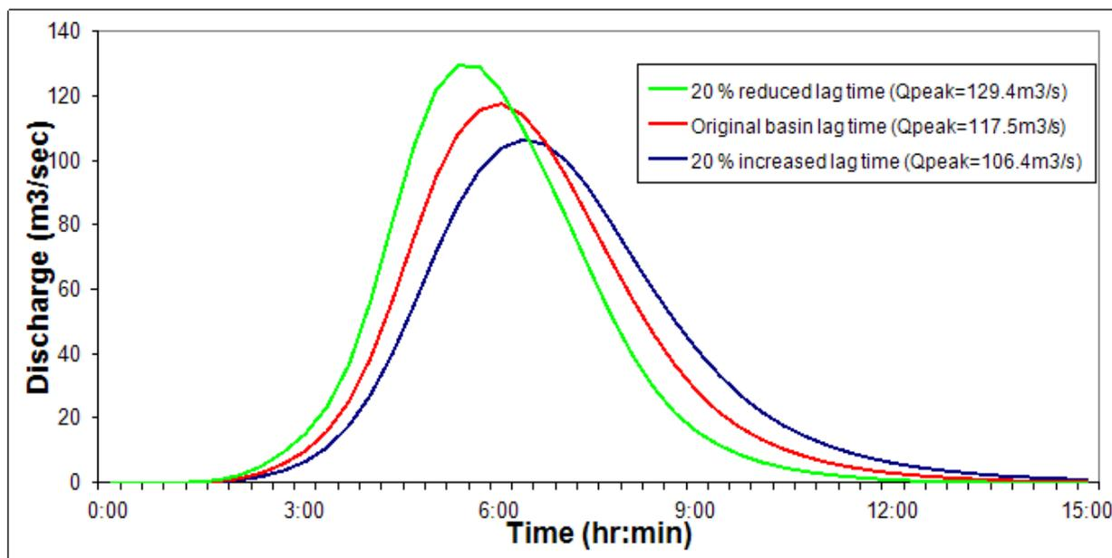
**Figure 28: Comparison of flood hydrograph resulting from 20 % increased and decreased lag times**
