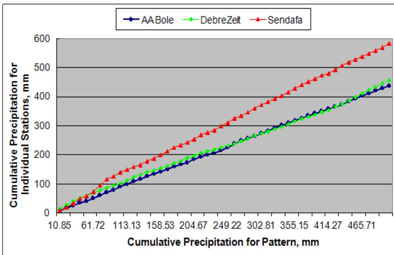
**Figure 21: Double Mass Curve for Precipitation Data**
