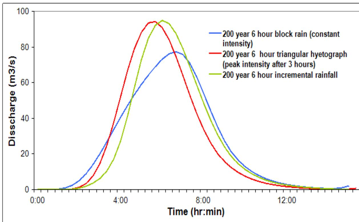
**Figure 38: Hydrographs resulting from 6 hr storms with three different rainfall patterns**
