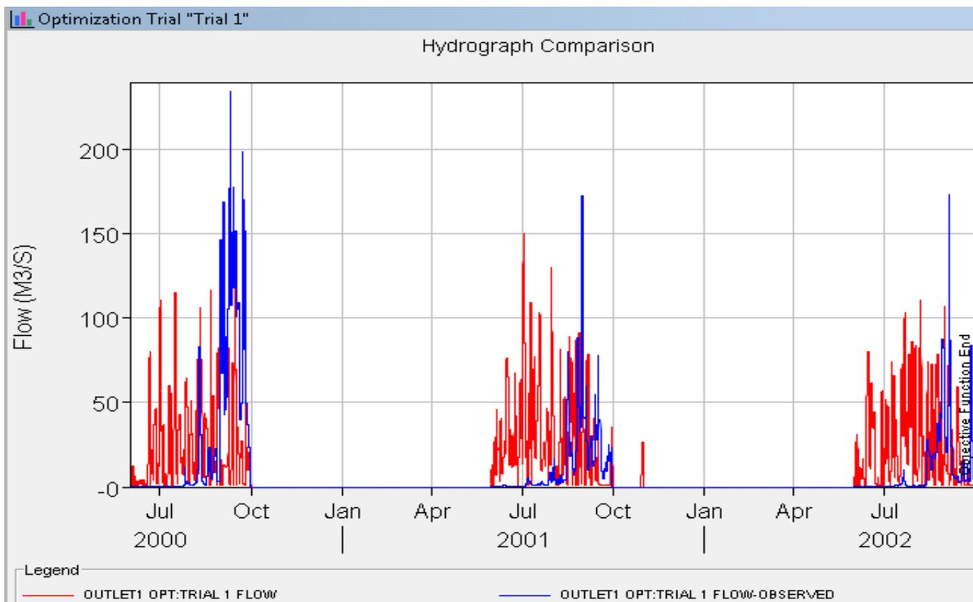
**Figure 29: Comparison of Simulated and Observed Flow**
