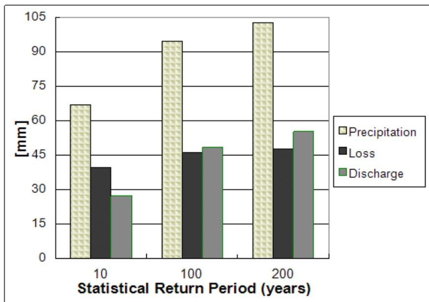
**Figure 35: Total precipitation, losses and discharge for return periods of 10, 100 and 200 years**
