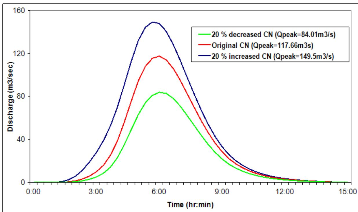
**Figure 27: Comparison of hydrograph resulting from 15% increased and decreased curve number**
