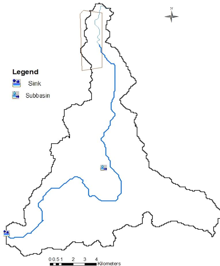
**Figure 24: Model Representation of the Study Watershed in HEC-HMS**
