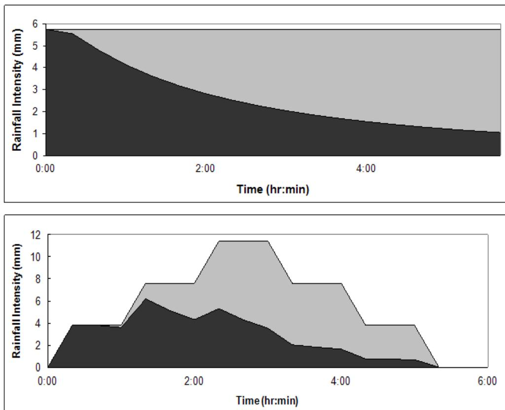
**Figure 37: Loss computation for 6 hr 200 year storms with three different intensity distributions**
