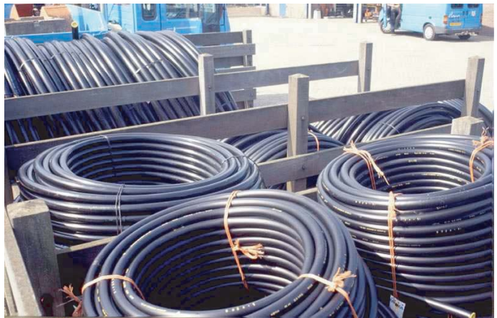
Figure 4.42. Stock of coiled PE pipes.
