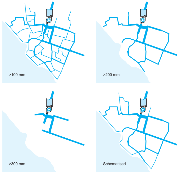
Figure 4.24. Example of network schematisation.
