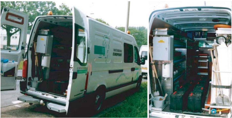
Figure 6.44. Mobile workshop for quick repair service.
