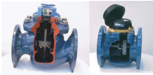
Figure 4.61. Inferential meters with vertical and horizontal axis.
