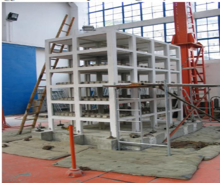
Test model on the 4 X 4 meter shaking table
