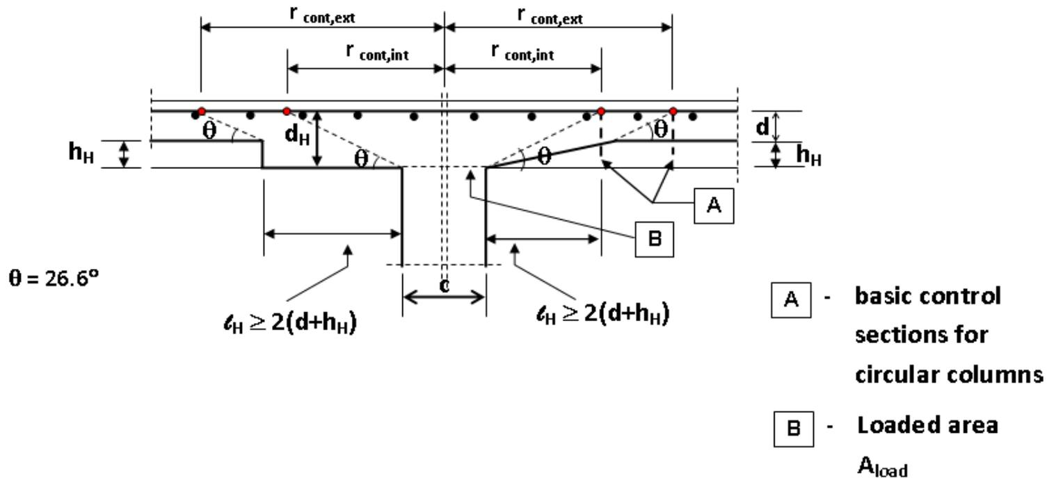
Fig: Slab with enlarged column head where  $l_H > 2(d+h_H)$
