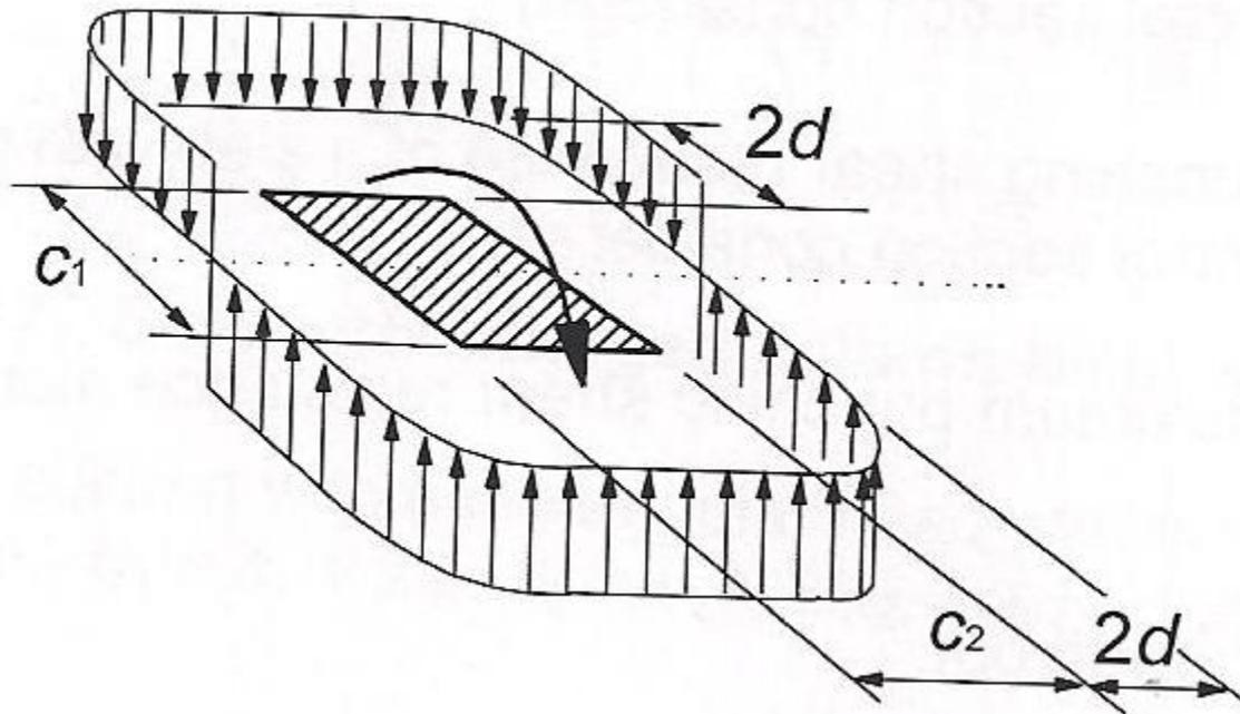
**Fig: Shear distribution due to an unbalanced moment at a slab-internal column connection**
