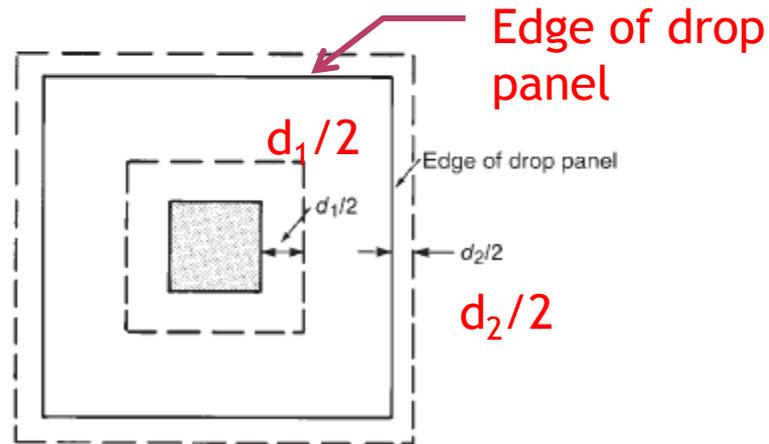
Fig. Critical sections in a slab with drop panels
