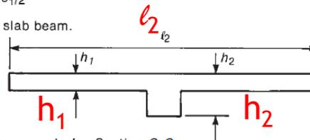
(c) Cross section used to compute  $I_1$ —Section C-C
