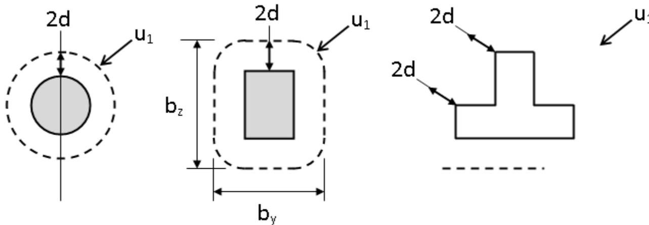
**Fig: Typical basic control perimeters around loaded areas**
