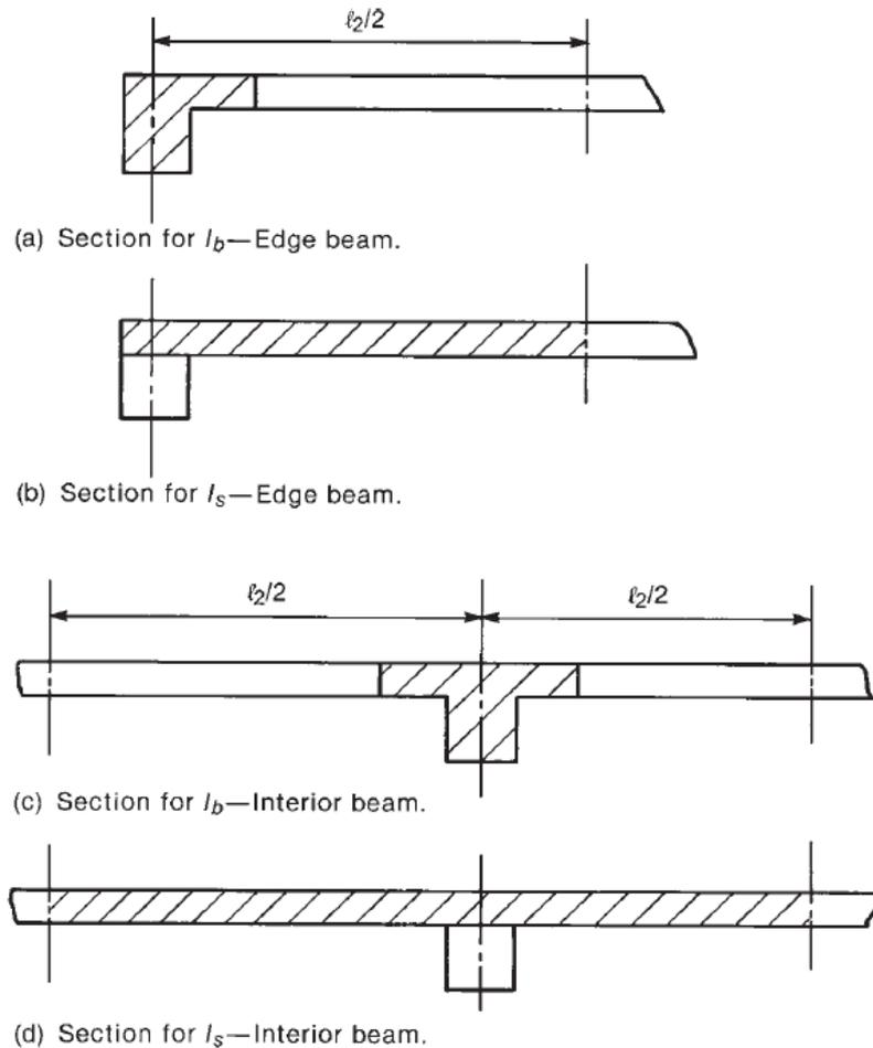
Fig. Beam and slab sections for calculations of  $\alpha_f$
