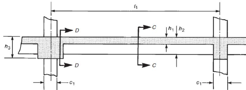
(a) Slab with beams in two directions.
