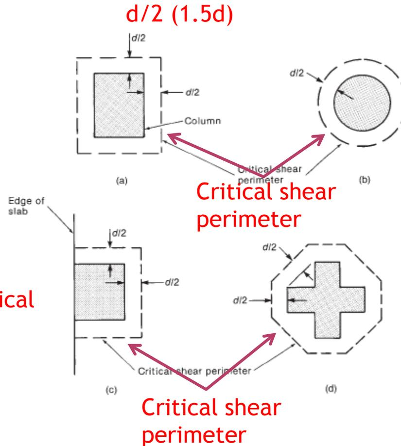
Fig. Location of critical shear perimeter
