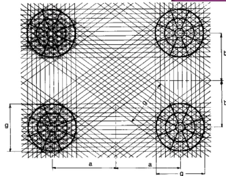
(b) Plan of reinforcement.
