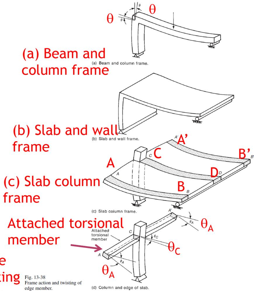
Fig. 13-38 Frame action and twisting of edge member
