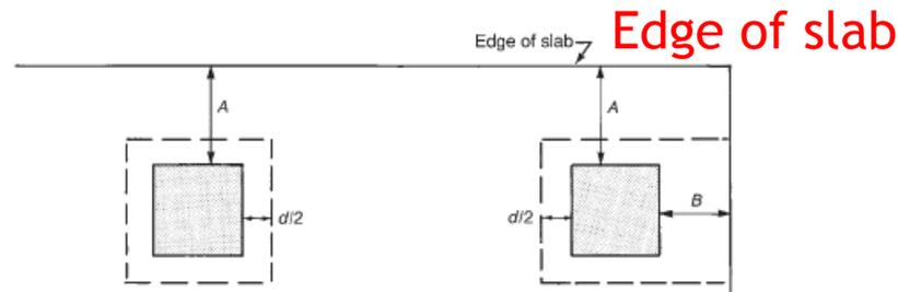
(c) Critical perimeter if A exceeds the greater of  $4h$  or  $2l_d$  but B does not
