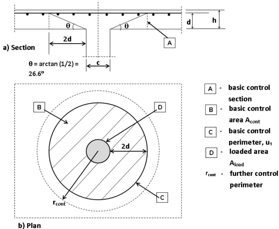
Fig: Verification model for punching shear at the ultimate limit state
