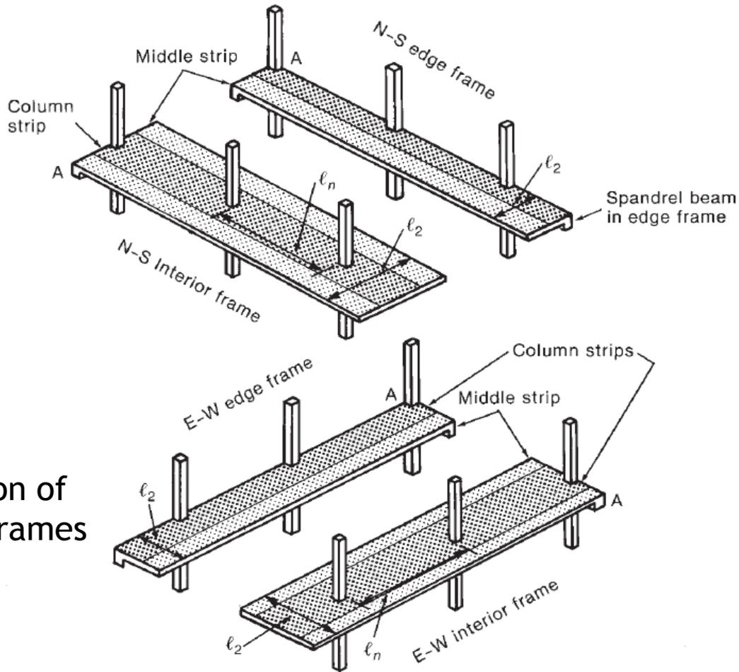
Fig: Division of slab into frames for design
