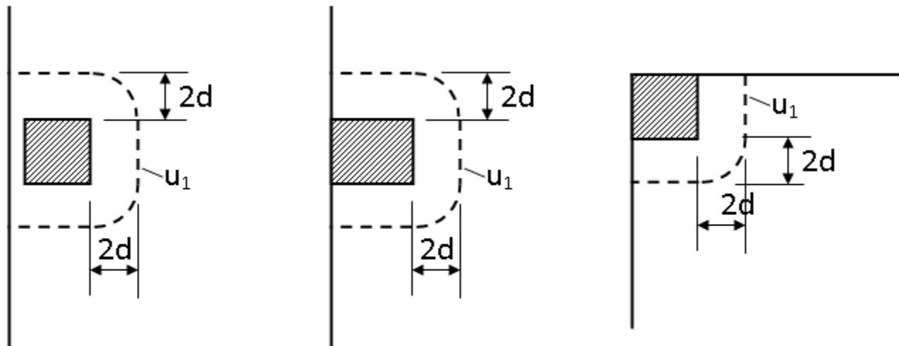
Fig: Control perimeters for loaded areas close to or at edge or corner
