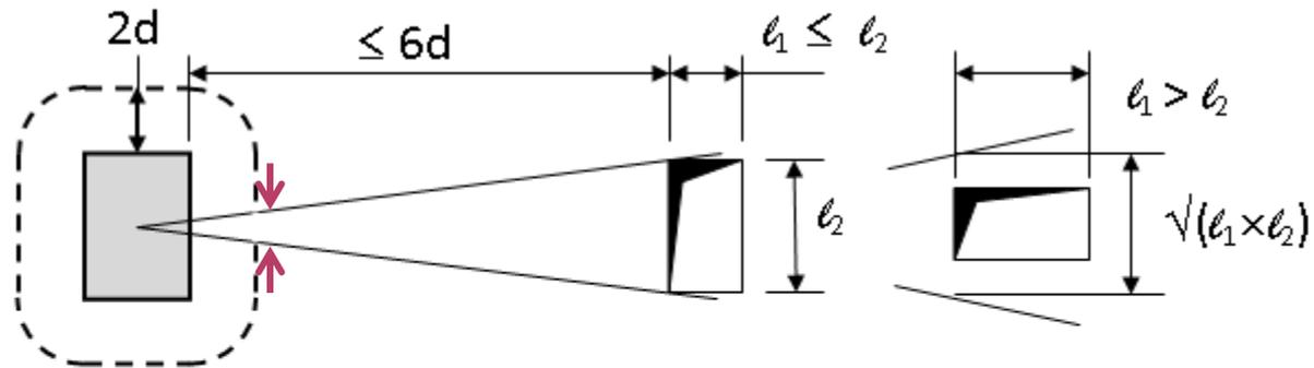
Fig: Control perimeter near an opening
