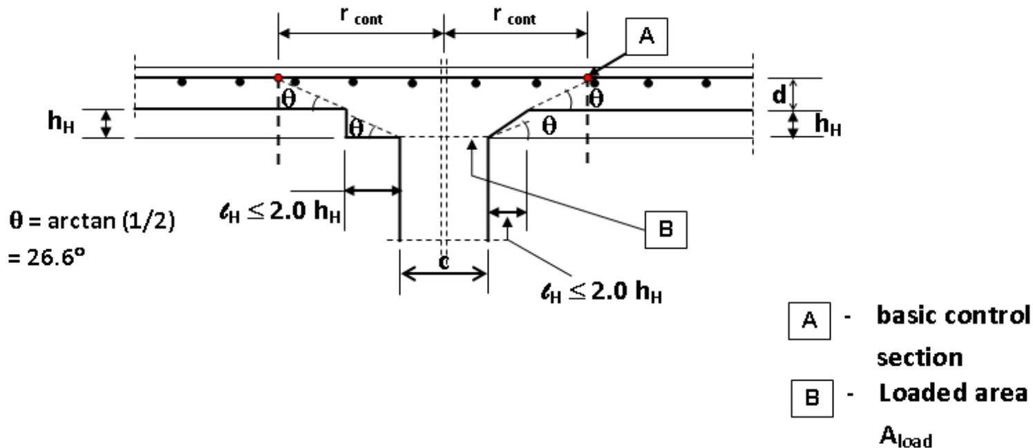
Fig: Slab with enlarged column head where  $l_H < 2.0 h_H$
